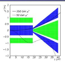
Polarity of the magnetic field is indicated by the blue/green colour of the iron poles of the magnets. The trajectories of a 350~GeV/c muon and 50~GeV/c muon are shown with a full and dashed line, respectively.
