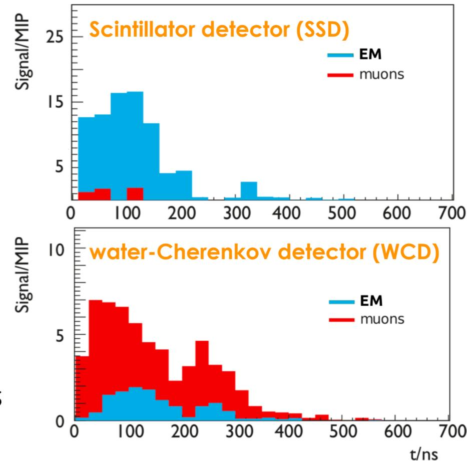
► Exploit the difference response of the two detectors to the electromagnetic and muonic showers components
