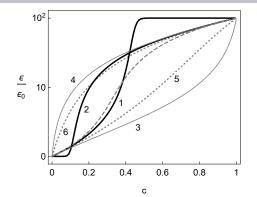
Figure: The concentration dependence of  $\varepsilon$  according to: the new low- (22) and high-concentration (23) rules (thick solid lines 1 and 2, respectively); Hashin-Shtrikman bottom and upper bounds (thin solid lines 3 and 4); CGA (10) (dashed line); original ABM low- (12) and high-concentration (14) rules (dotted lines 5 and 6). The only parameter used  $\varepsilon_1/\varepsilon_0 = 10^2$ .
